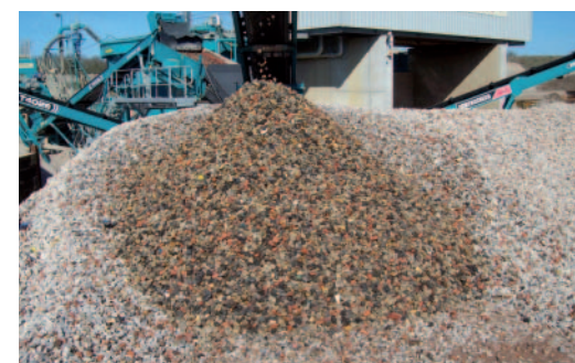
Recycled, washed aggregate can now be used in ready-mixed concrete.
