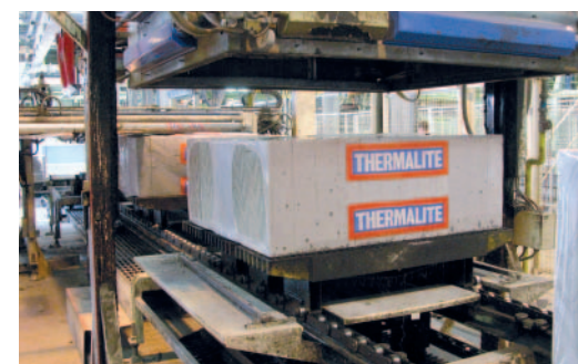
Cement substitutes are used in the manufacture of Thermalite blocks.
