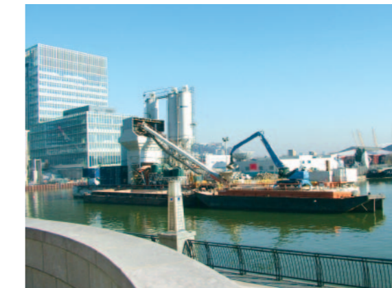
Hanson's floating concrete plant at Wood Wharf in the heart of London's Docklands is keeping thousands of lorries off the capital's roads
